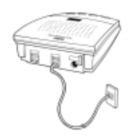
If you wish to connect both the DTAM and a telephone to the telephone line, simply use the two way splitter supplied. Plug the splitter into the telephone wall socket then plug the DTAM into one side of the splitter and the phone into the other side.
